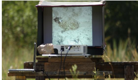
Figure 5. To increase the scope of environmental conditions in our laboratory testing, we adapted an evaluation technique from human biometrics: semi-synthetic models [10, 23]. Semi-synthetic models are derived from individual source object data, but also capture important conditions such as weather and atmospheric effects that impact long-range data for animal population studies. We re-imaged our data set outdoors at 100M on a sunny day, with a setup that consisted of a 4000 ANSI lumens projector with a resolution of 1024 \times 768 projecting into a custom built screen, imaged by a Canon EOS 7D Camera with a Canon 2 \times adapter and a Sigma 800mm F5.6 lens. This is an example image of our setup; for evaluation, we crop the image and pass it to the classifiers.
