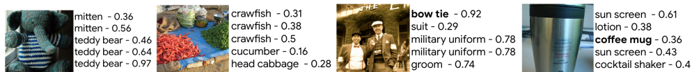
Figure 4: ImageNet trained on ResNet-v2-50: Sample predictions from 5 independent training runs and the prediction probabilities. True label is highlighted in the predictions. Despite all the runs achieving a top-1 accuracy of around 76%, individual predictions of these models can vary dramatically, highlighting the necessity of having methods with more reproducible predictions and less churn. Note that even when the independent runs predict the true label, their prediction probabilities vary significantly.
